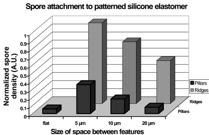
Figure 5: Spore attachment to patterned silicone elastomer. Features were 5 μm high.
