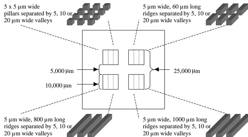
*Figure 1: Layout of the micro-patterned substrate etched to 1.5  $\mu\text{m}$  or 5  $\mu\text{m}$  depth. There were four 1  $\text{cm}^2$  main areas each with the feature type indicated in the diagram. Each main area was subdivided into three smaller 1/3  $\text{cm}^2$  areas with either 5, 10 or 20  $\mu\text{m}$  spacing between features.*
