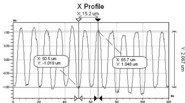
*Figure 3: 5000 cSt, 20 wt% oil modified elastomer wiped with toluene immediately before imaging. A 2-dimensional profile WLIP image sliced perpendicular to the long axis of the 5  $\mu\text{m}$  ridges separated by 5  $\mu\text{m}$  valleys. The variation in valley and peak heights can be clearly seen as well as the variable amplitude ranging from 1.7 to 2.5  $\mu\text{m}$ .*
